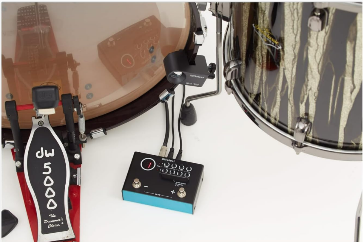
Image: A close-up view of the Roland TM-1 module on the floor next to a drum kit, showing its connections to drum triggers and a foot pedal.
