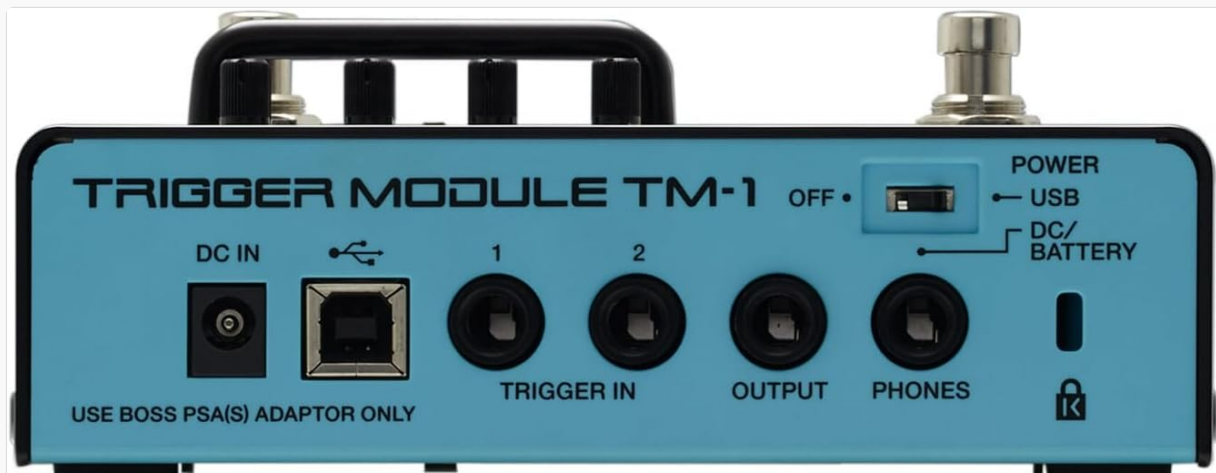
Image: Rear view of the TM-1 module, highlighting the DC IN, USB, Trigger In (1 & 2), Output, and Phones jacks. The power switch is visible, indicating USB or DC/Battery power options.
