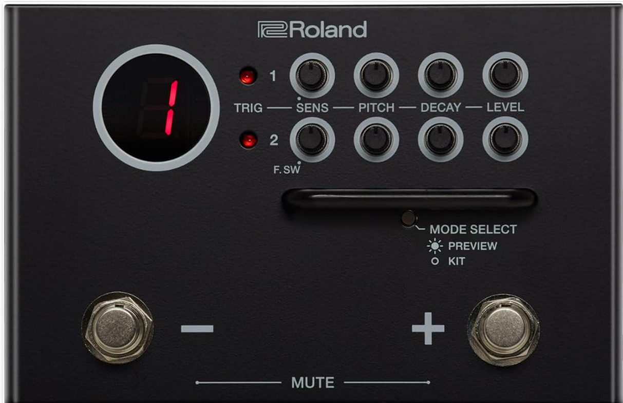
Image: Front panel of the TM-1 module, displaying the large LED display, Trigger 1 and 2 input indicators, and control knobs for SENS (Sensitivity), PITCH, DECAY, and LEVEL for each trigger. Also visible are the MODE SELECT switch (Preview/Kit) and the MUTE footswitches.
