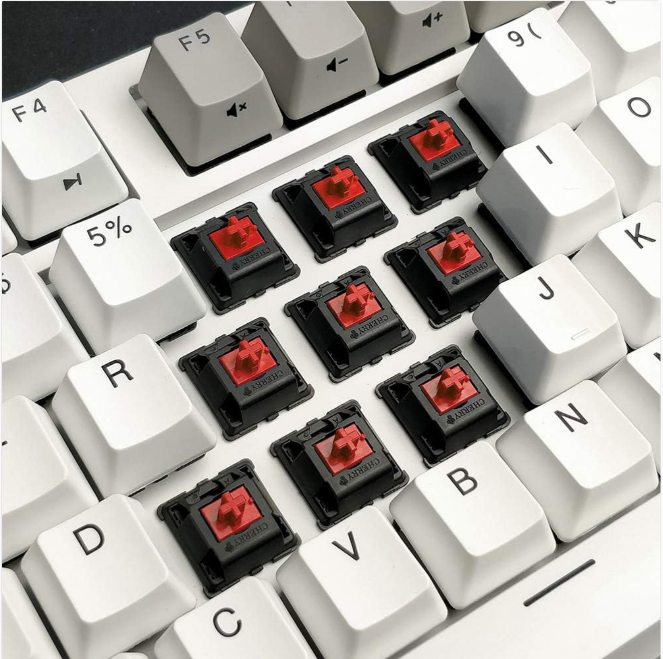
Image: A close-up view of the Cherry MX Red mechanical switches, visible after removing some keycaps.
