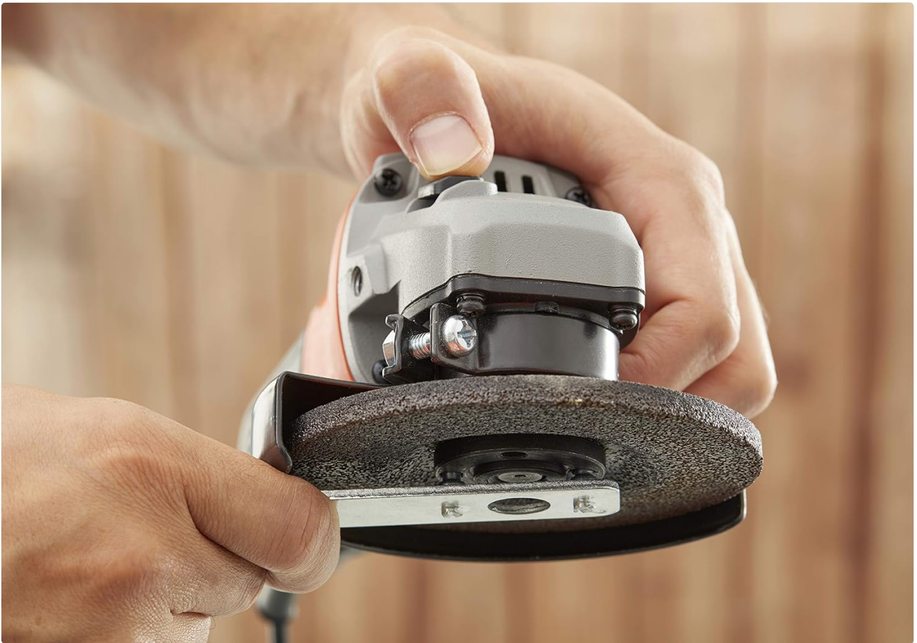
Figure 3: Illustrates the process of changing a grinding disc using the spindle lock and spanner wrench.
