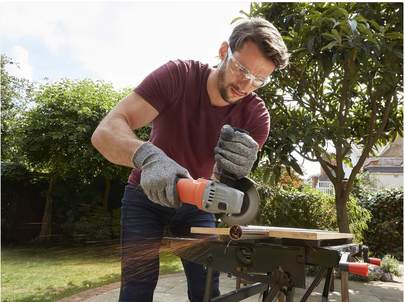
Figure 5: Demonstrating grinding a metal pipe with the angle grinder. Note the sparks and safety precautions.
