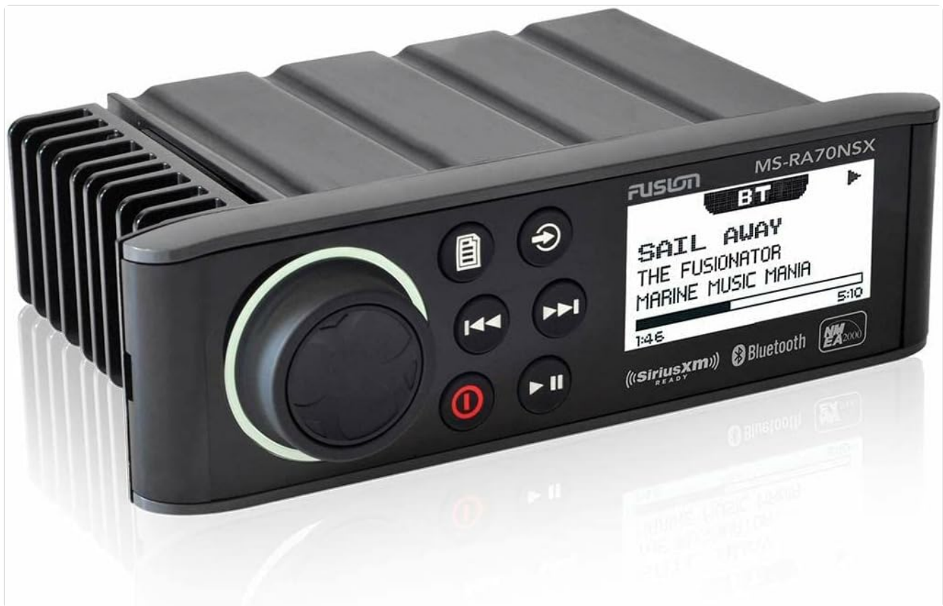
Figure 4.1: Front view of the Fusion MS-RA70NSX Marine Entertainment System, showing the display, rotary knob, and control buttons.
