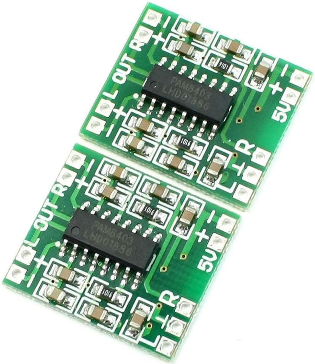
Image 1.1: Two PAM8403 Mini Amplifier Modules. These small green circuit boards feature the PAM8403 chip and various surface-mount components, designed for stereo audio amplification.
