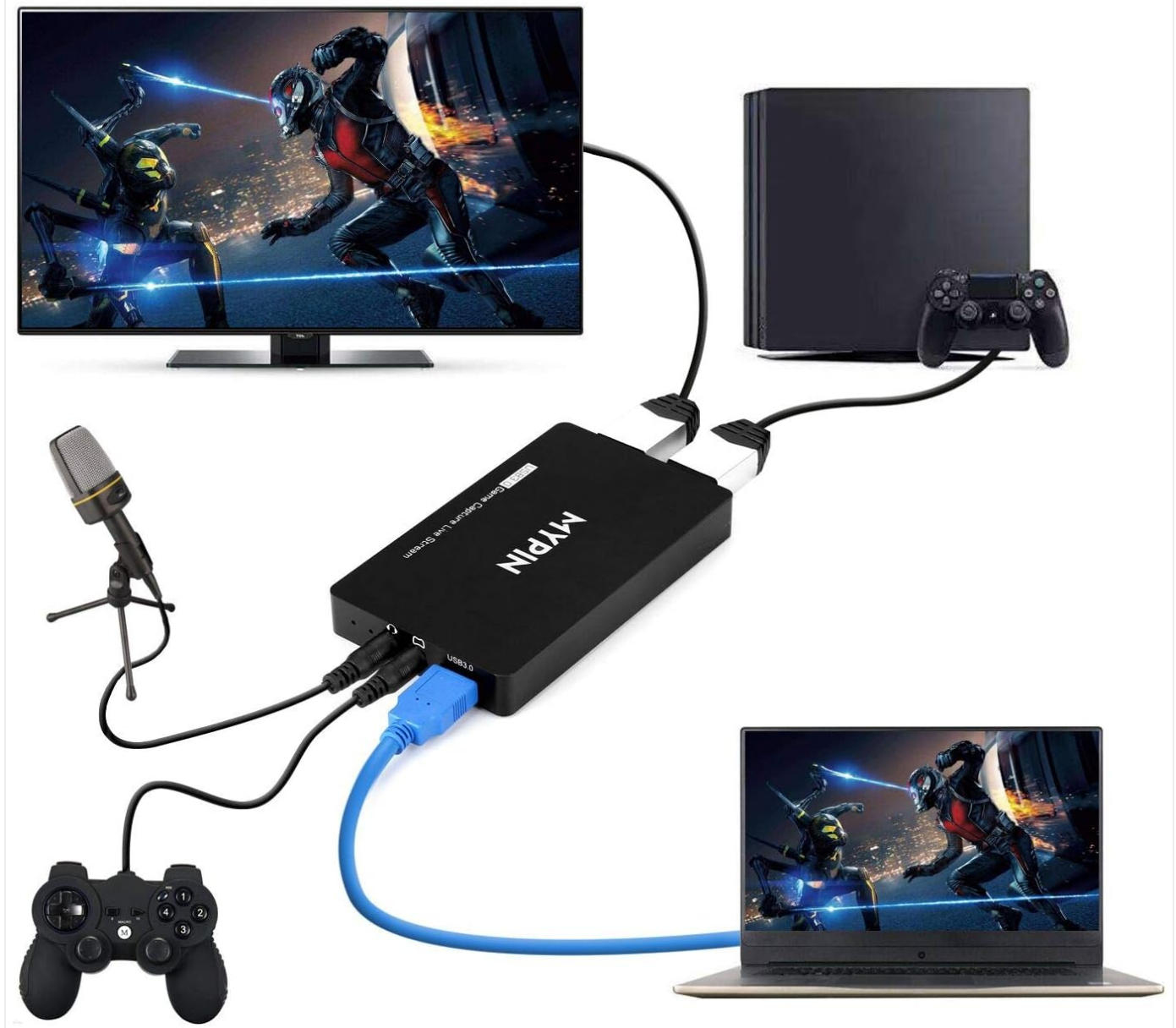
Image 4.2: Illustration of a live streaming setup, showing the capture card connecting a console to a PC for streaming and a TV for passthrough viewing.
