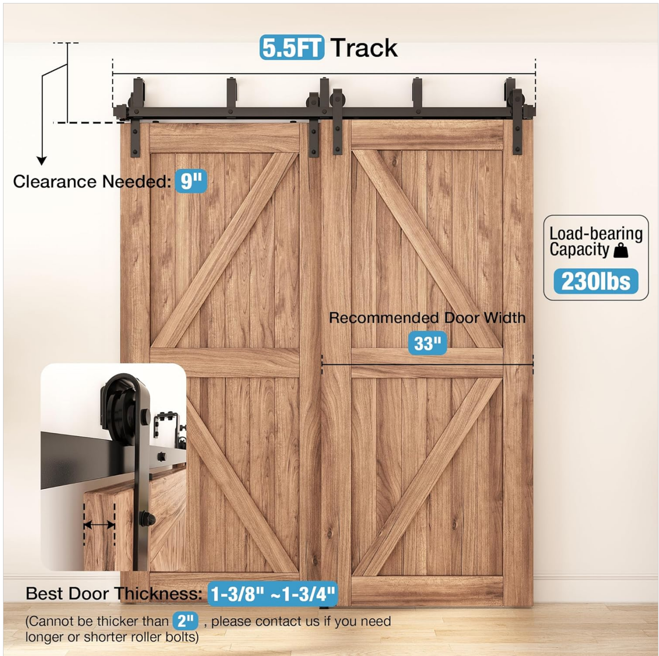
Figure 1: Key dimensions and requirements for installation.
