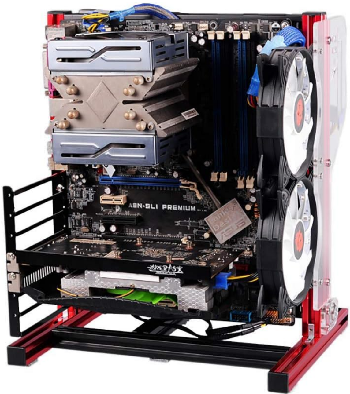
Figure 1: Fully assembled PC Test Bench with a motherboard, CPU cooler, graphics card, and fans installed, demonstrating its open-frame design.
