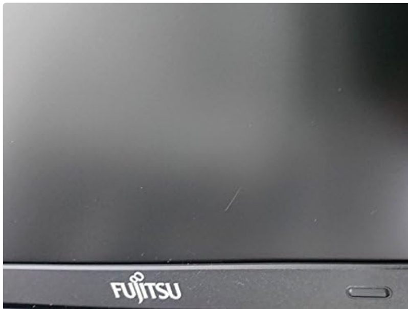
Figure 4: Close-up of the screen showing a scratch.
