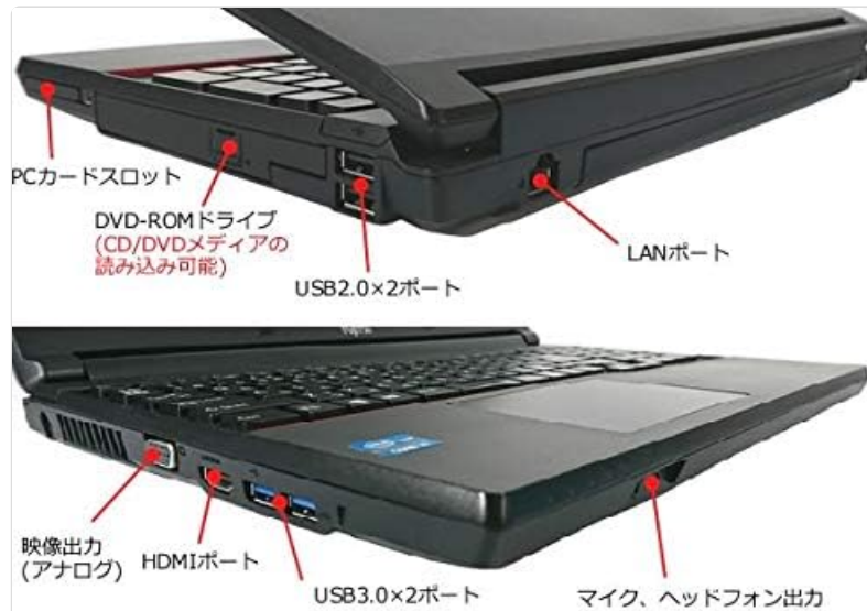
Figure 2: Port layout of the Fujitsu LIFEBOOK A573/G.
