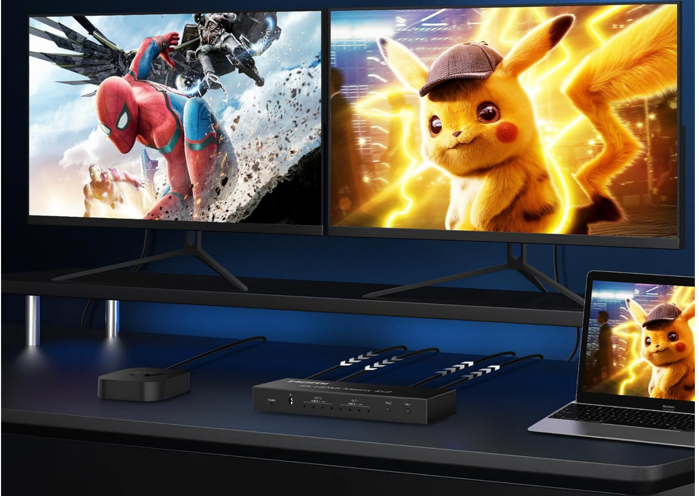
Example of Matrix Mode setup, where two different sources are displayed on two different screens.
