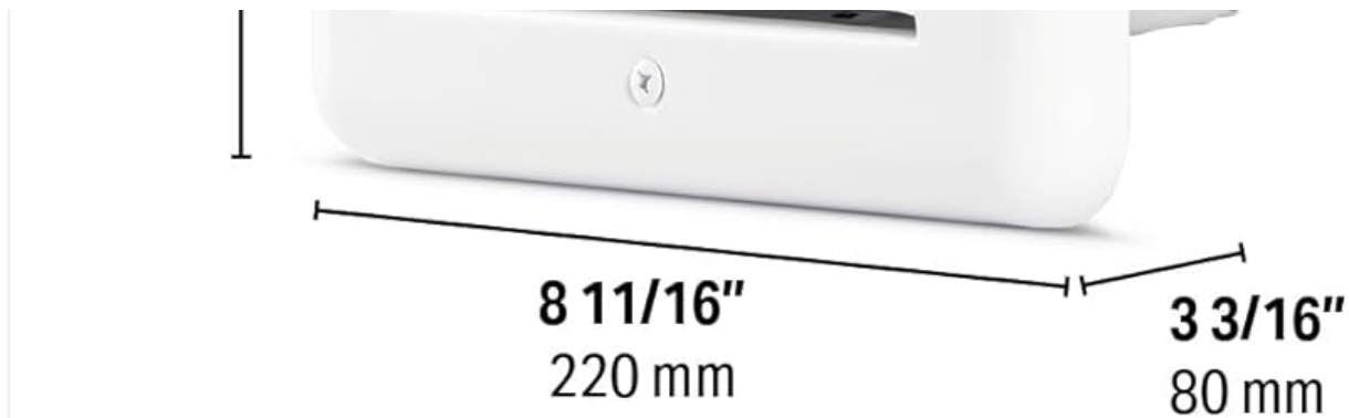
Diagram showing the dimensions of the Stelpro pulsair RWF0502W wall fan heater: 17 1/8 inches (435 mm) height, 8 11/16 inches (220 mm) width, and 3 3/16 inches (80 mm) depth.
