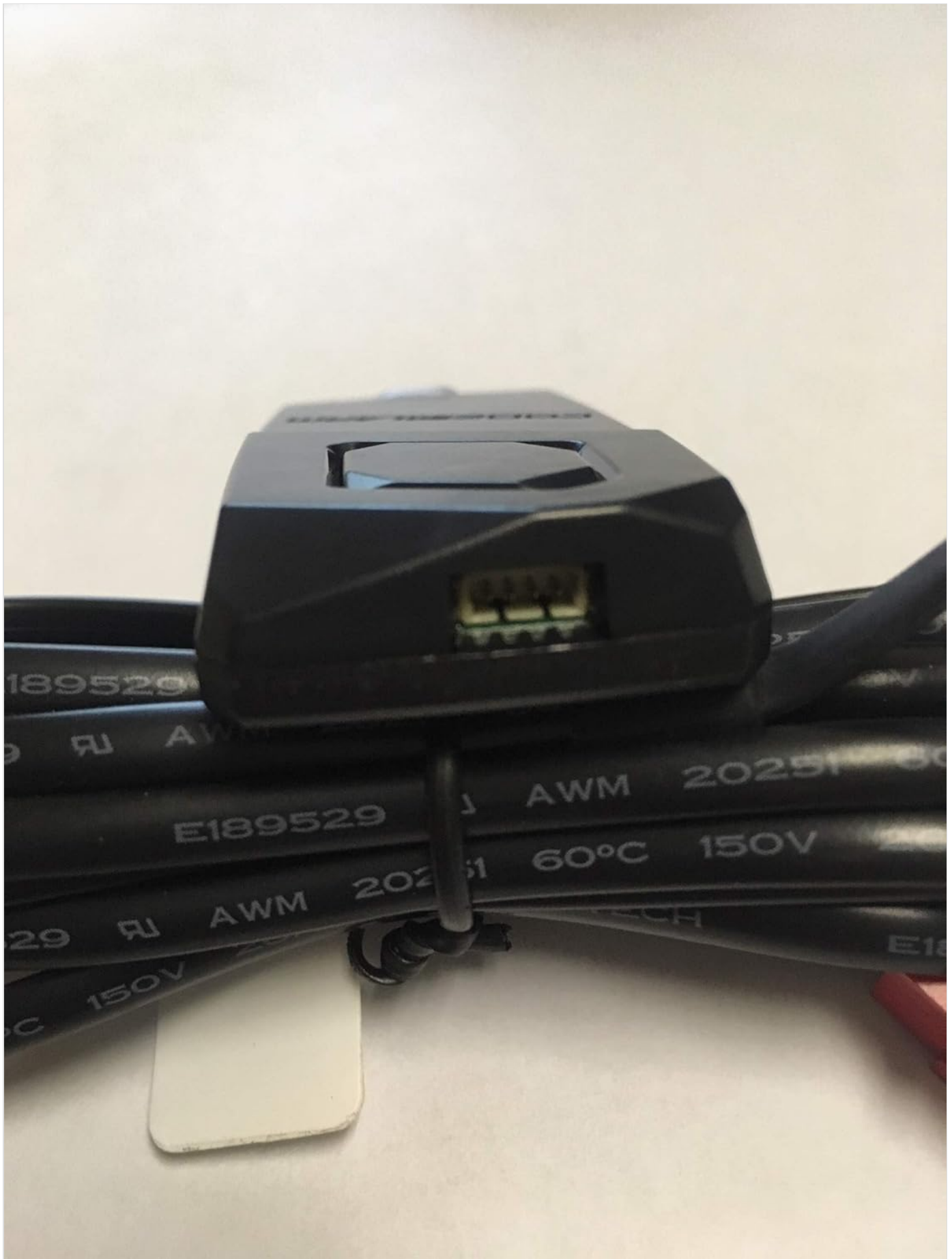
Image 3: Detailed view of the Code Alarm 41800640 antenna unit, showing the connection port where the 41203880 cable attaches. The cable is coiled next to the antenna.
