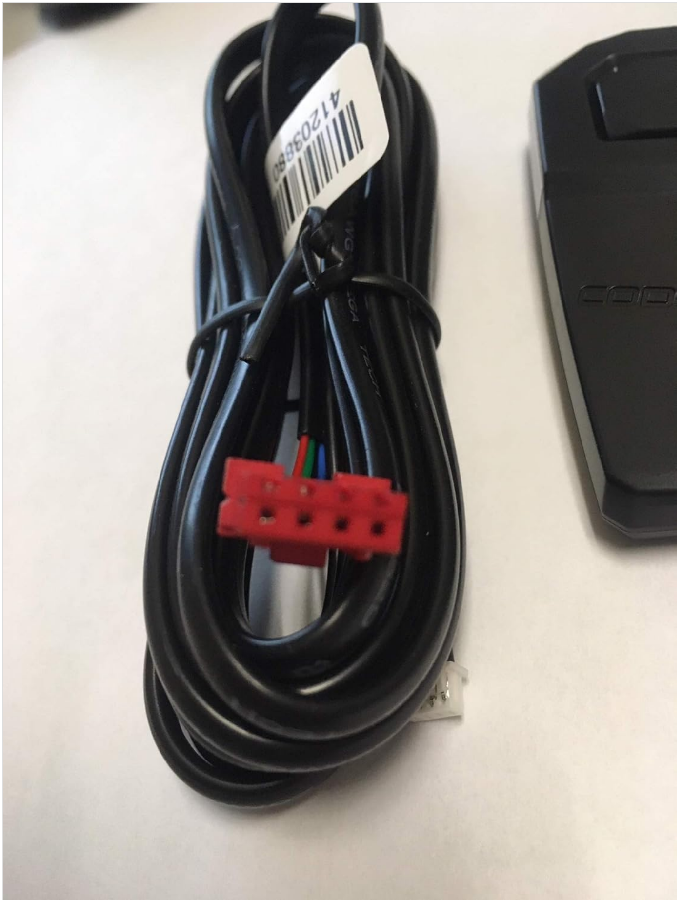
Image 1: The Code Alarm 41800640 2-Way Replacement Antenna and 41203880 Cable. This image shows the antenna unit and the coiled cable with its connectors.
