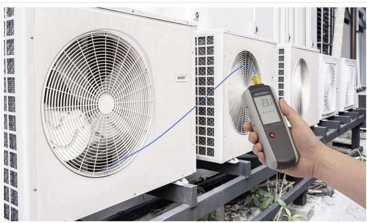
Figure 6.1: The VOLTcraft TP-202 Type K Air Sensor connected to a compatible handheld thermometer, measuring the temperature of an air conditioning unit.
