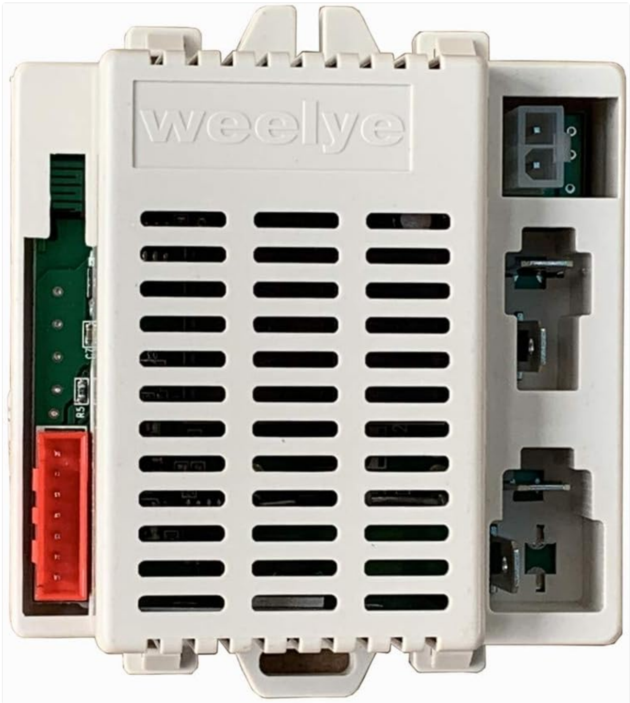
Image 2.3: The new style weelye receiver, which is functionally equivalent to the old style.
