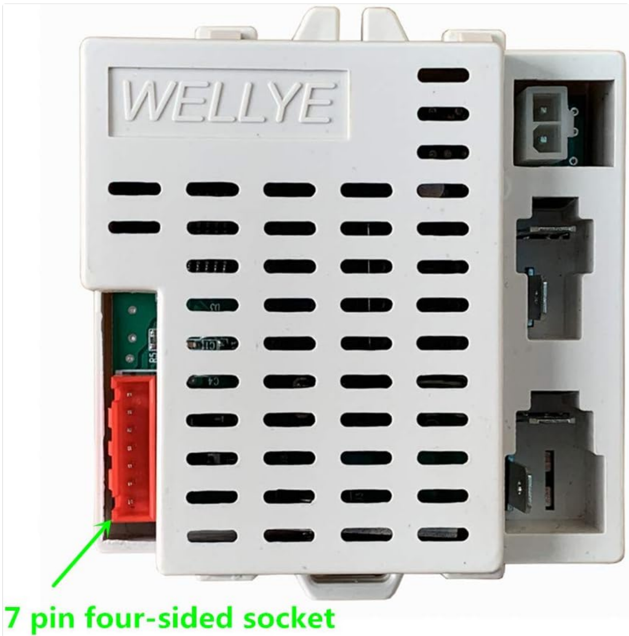
Image 2.2: Close-up of an old style receiver, highlighting the 7-pin four-sided socket for connection.
