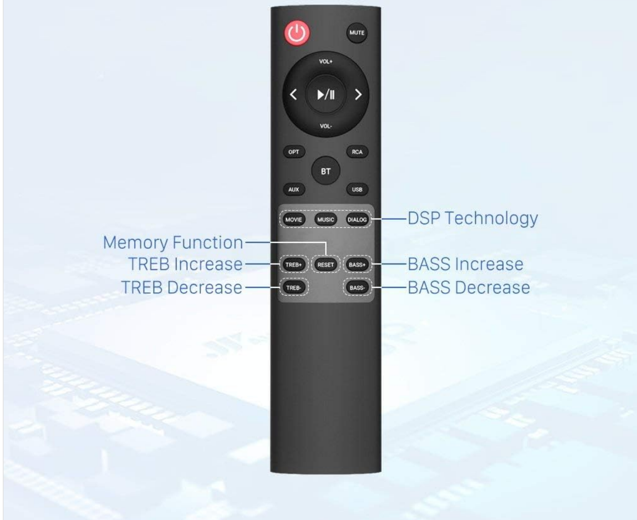
Image 3.2: Detailed view of the remote control, highlighting buttons for Memory Function, Treble Increase/Decrease, Bass Increase/Decrease, DSP Technology (Movie, Music, Dialog), and input selection (OPT, RCA, BT, AUX, USB).
