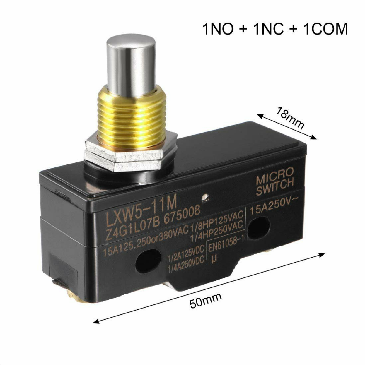
Figure 2: Dimensions of the uxcell LXW5-11M Micro Limit Switch. This image illustrates the length (50mm) and width (18mm) of the switch body, and indicates the 1NO + 1NC + 1COM contact configuration.
