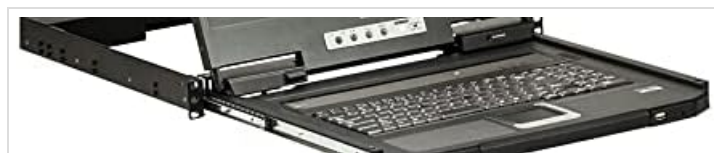
Figure 3: The ATEN CL3700NW console with the keyboard and touchpad tray extended for use.
