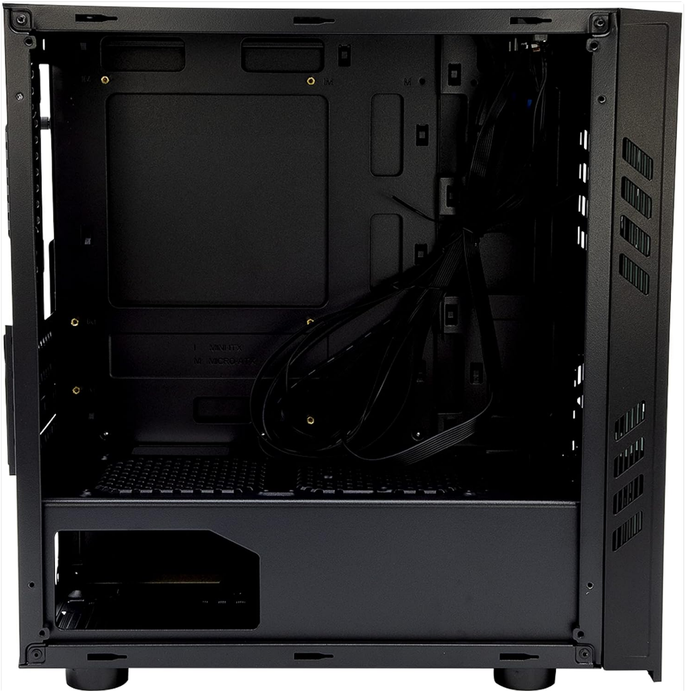
Image: Interior view of the Yeyian Kalt 1101 PC case, showing the motherboard mounting area and cable routing cutouts.
