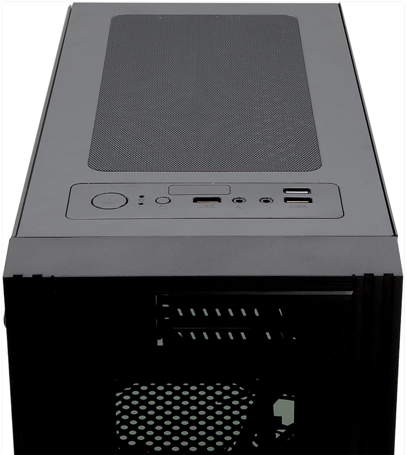
Image: Top view of the Yeyian Kalt 1101 PC case, showing the power button, reset button, USB 3.0, and USB 2.0 ports.
