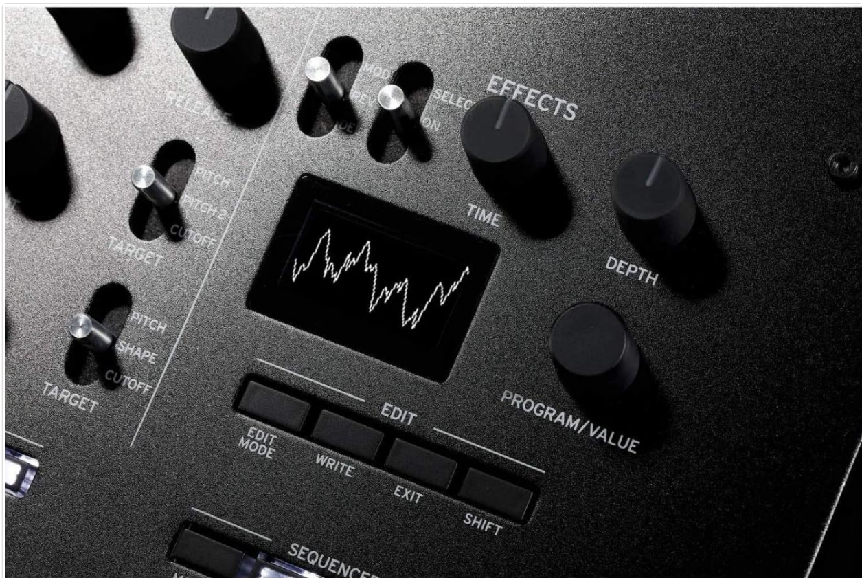
Figure 4: Effects and Display. This image focuses on the effects section and the OLED oscilloscope display, which visually represents the waveform as it is being shaped by the various parameters.
