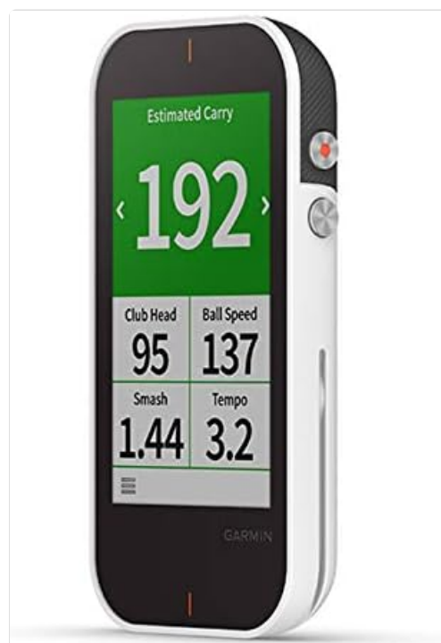
Figure 6: Garmin Approach G80 showing estimated carry distance, club head speed, ball speed, smash factor, and tempo.
