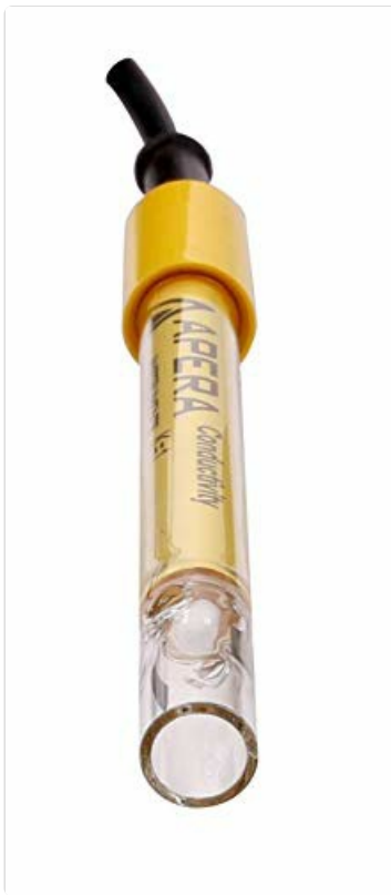
Figure 4: Close-up view of the platinum glass-body conductivity electrode tip, which requires careful handling and proper storage.
