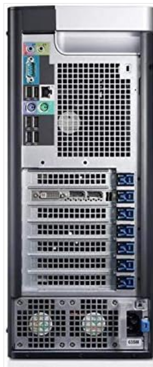
Figure 2: Rear view of the Dell Precision T3600 Workstation. This image shows the back panel with various input/output ports including USB, audio, network, and video outputs (DVI).
