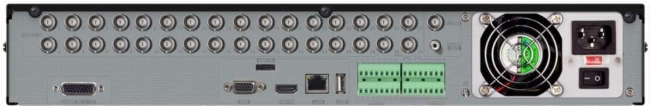
Figure 2: Rear view of the Titanium ED8432H5-D DVR. This panel includes 32 BNC video input ports, RCA audio inputs/output, VGA and HDMI video outputs, Ethernet port, USB ports, RS485 terminal, and the power input with an on/off switch.
