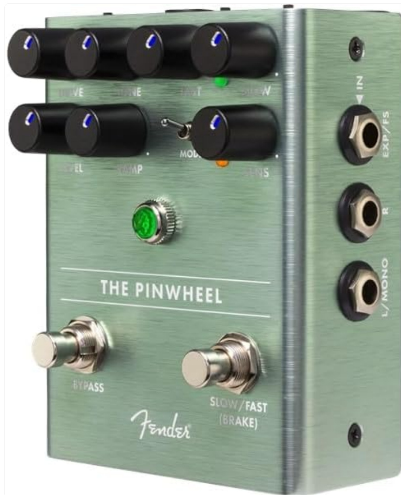
Figure 2: Side view of the pedal, illustrating the input and output jacks for mono and stereo connections.
