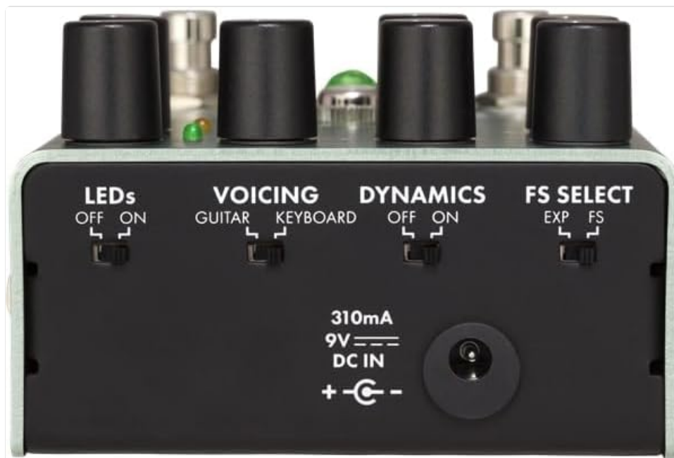
Figure 3: Rear view of the pedal, detailing the utility switches and power input.
