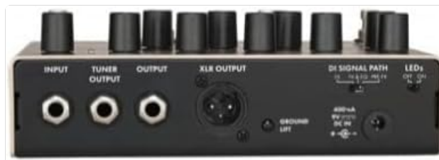
Figure 4.2: Rear panel connections of the Fender Downtown Express Bass Multi-Effect Pedal.
