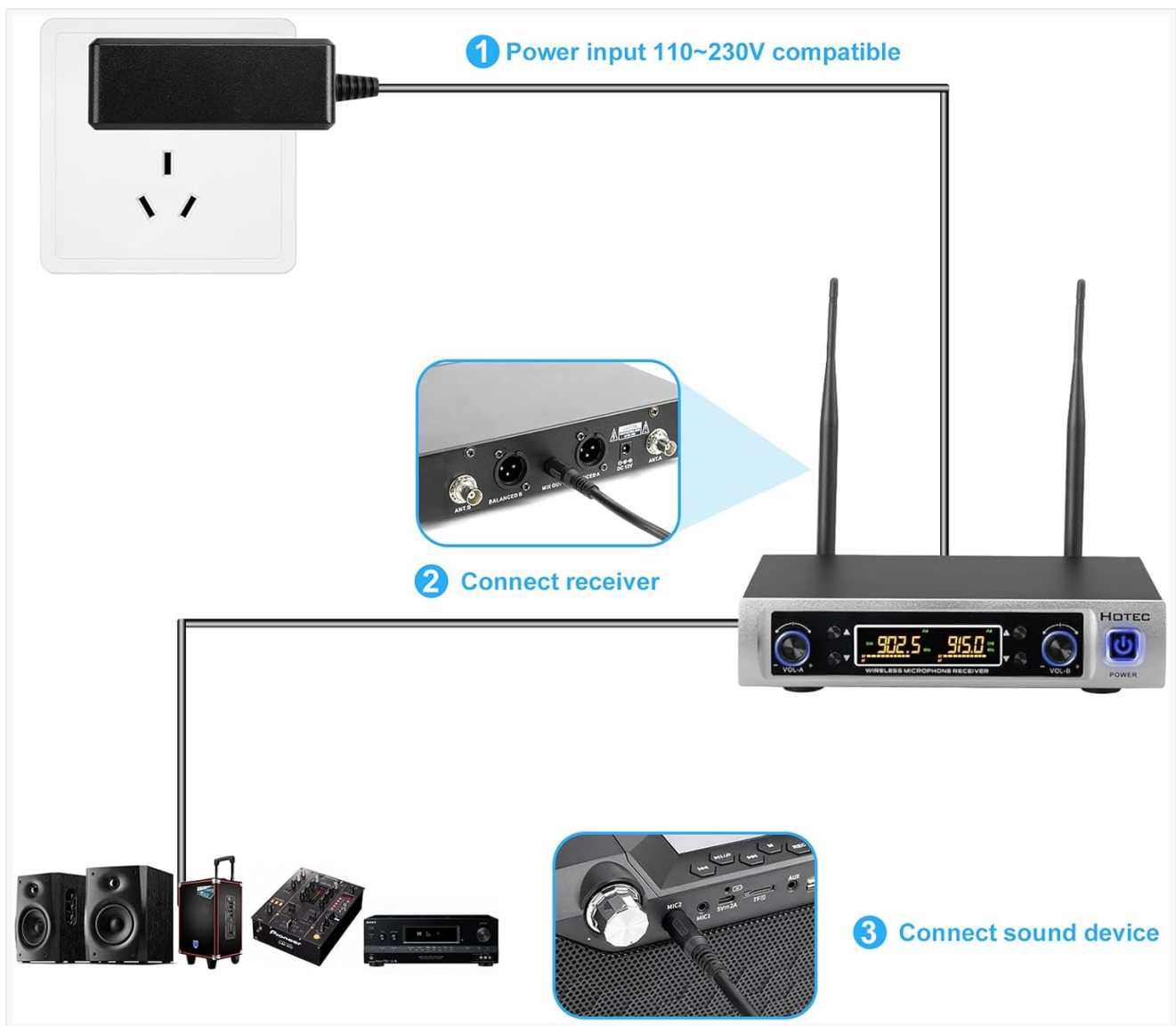
Figure 3.1: Visual guide for connecting the wireless microphone system to a sound device.
