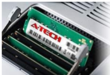
Image: A memory module fully seated and secured in a laptop's SO-DIMM slot.
