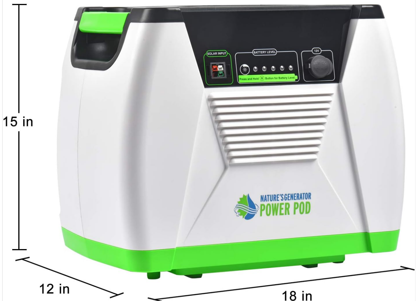
Figure 4: Dimensions of the Nature's Generator Power Pod, approximately 15 inches high, 12 inches wide, and 18 inches deep. It weighs 92 lbs and contains an AGM Sealed Lead Acid battery with 100Ah (1200Wh) capacity.
