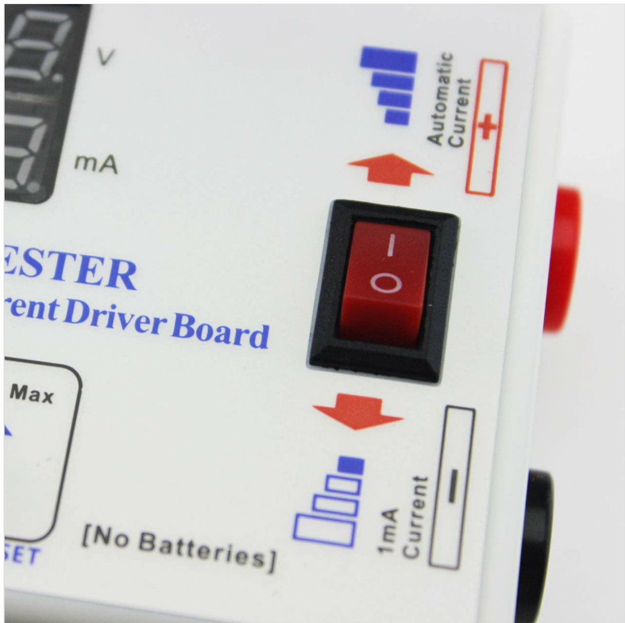
Figure 3: Detail of the power switch and current selection switch on the tester.
