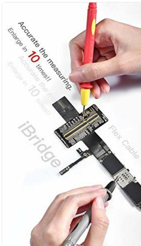
**Figure 4.1:** A close-up view demonstrating the use of multimeter probes on the extended test points of an iBridge flex cable. This highlights the ease of access for precise measurements.
