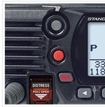
Figure 6: Power button (red) and the spring-loaded DISTRESS button.
