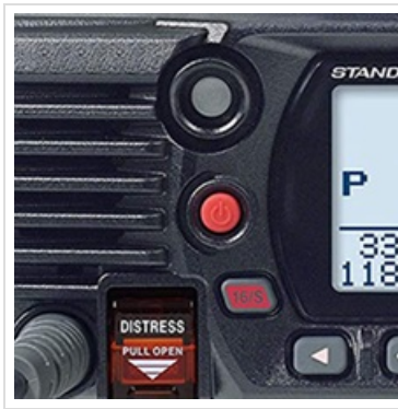
Figure 9: The red spring-loaded DISTRESS button for emergency calls.
