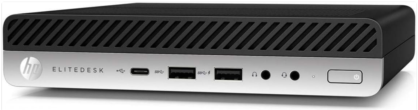
Figure 1: Front view of the HP EliteDesk 800 G4 Mini Desktop, showing the power button, USB-C port, USB 3.1 ports, and audio jacks.
