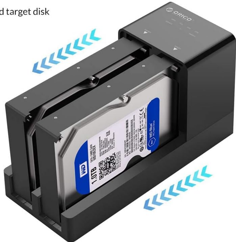
Figure 5.2: Illustrates the three steps for an offline clone: 1. Power on, insert source and target disk. 2. Press button. 3. Automatically copy. Progress indicators (25%, 50%, 75%, 100%) are shown. For more information on the Western Digital drives shown, visit http://qr.wdc.com/wdblue .
