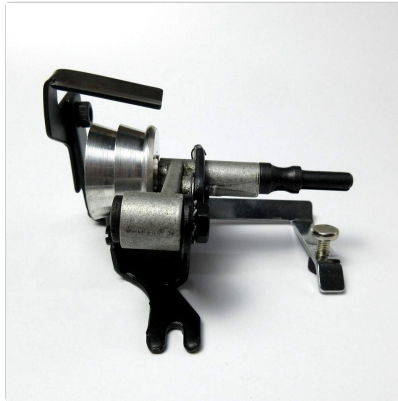
Figure 3: Another side view of the Bobbin Winder Assembly, showing the full length of the bobbin spindle and the adjustment screw.
