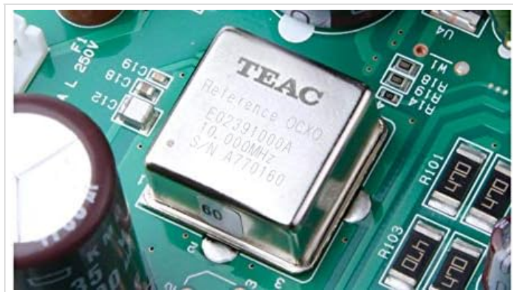
Figure 2: Internal view showing the high-precision TEAC Reference OCXO clock, contributing to accurate audio timing.
