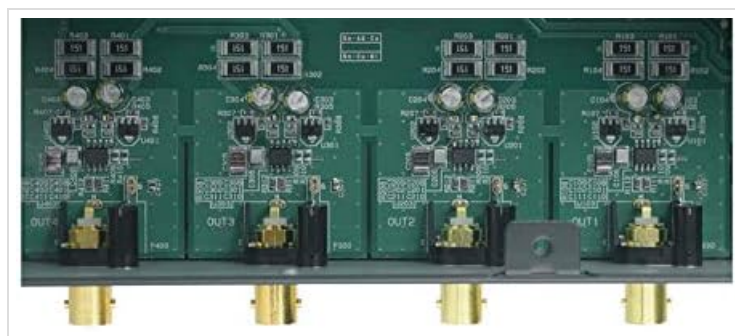
Figure 3: Internal view of the TEAC-HCLD buffer amplifier circuits, designed for enhanced acoustic expression.
