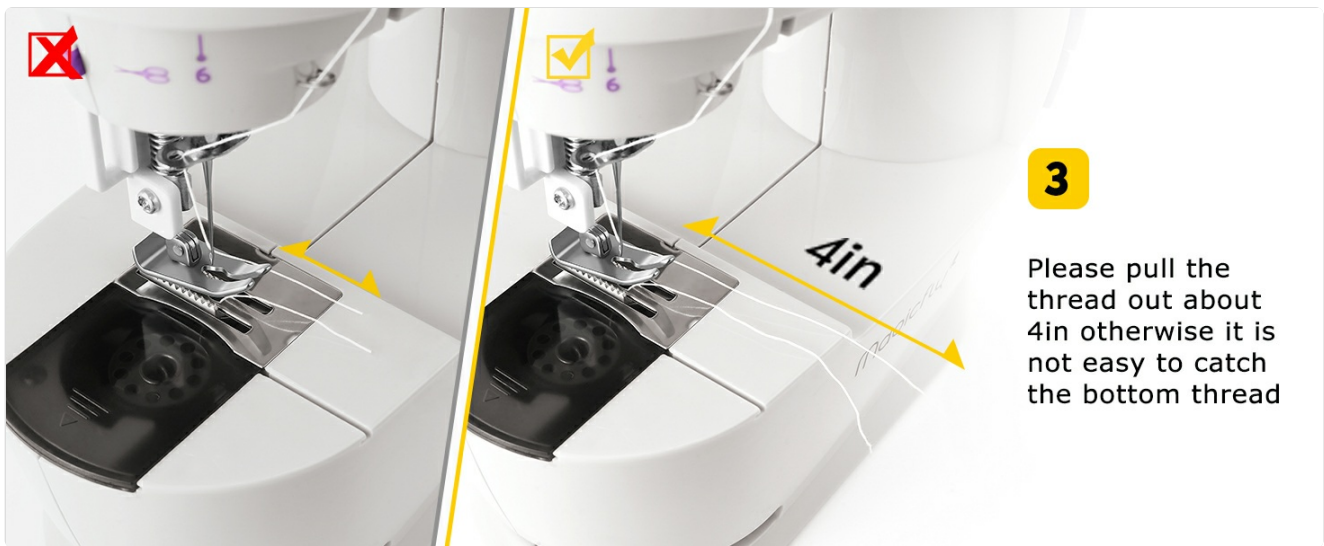
Image: Ensure sufficient lower thread is pulled out (approximately 4 inches) to allow the upper thread to catch it properly.
