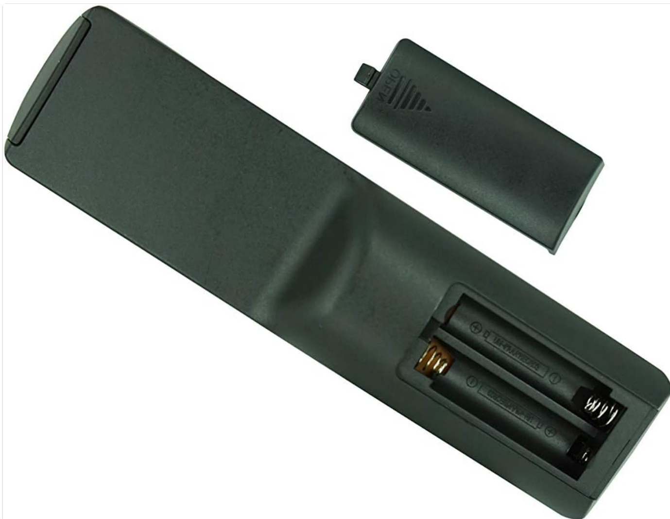
Image: Back view of the remote control with the battery cover removed, illustrating the correct insertion of two AA batteries.
