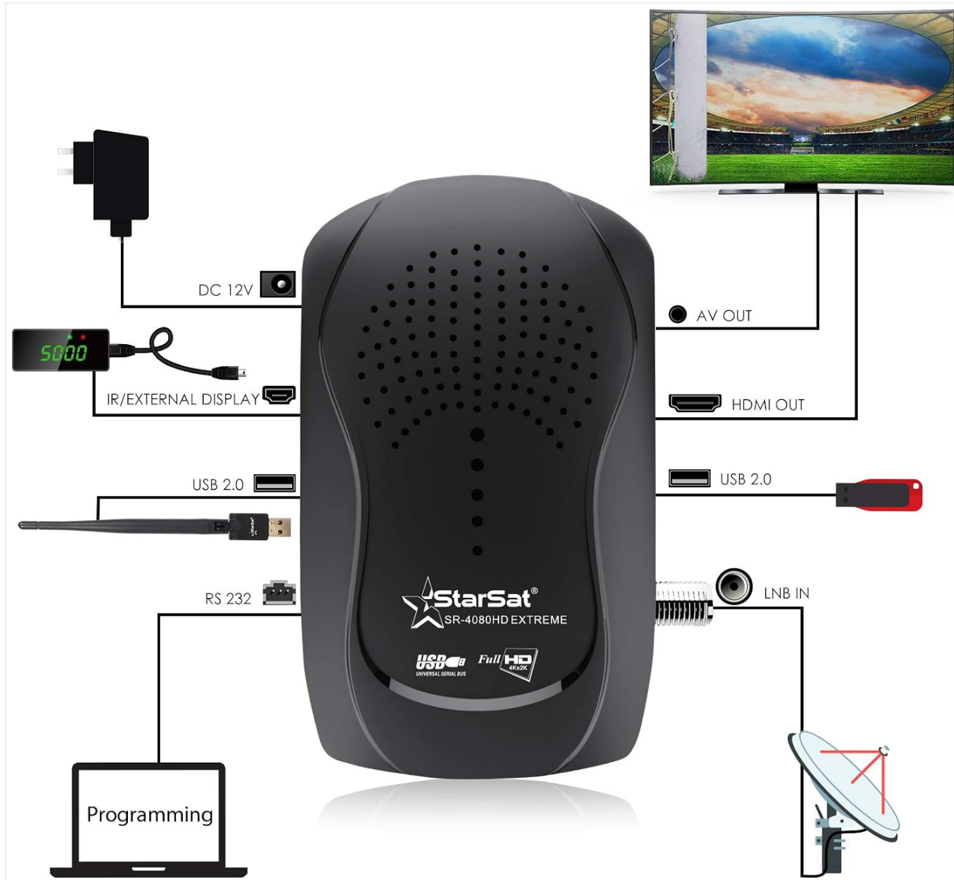
Figure 4.2: Connection diagram illustrating the various ports and their typical connections. This includes DC 12V power input, IR/External Display port, USB 2.0 ports, RS 232 port for programming, LNB IN for satellite dish connection, HDMI OUT, and AV OUT.
