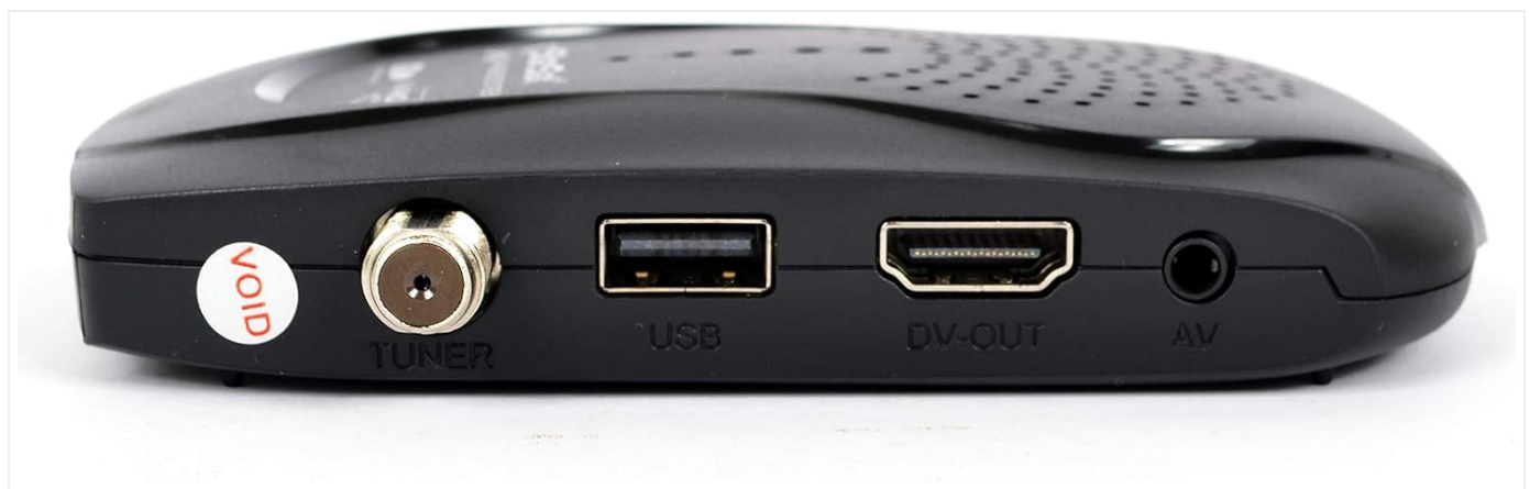
Figure 4.3: Close-up view of the rear ports on the Star Sat SR-4080HD Extreme, showing the Tuner (LNB IN), one USB port, DV-OUT (HDMI), and AV port.
