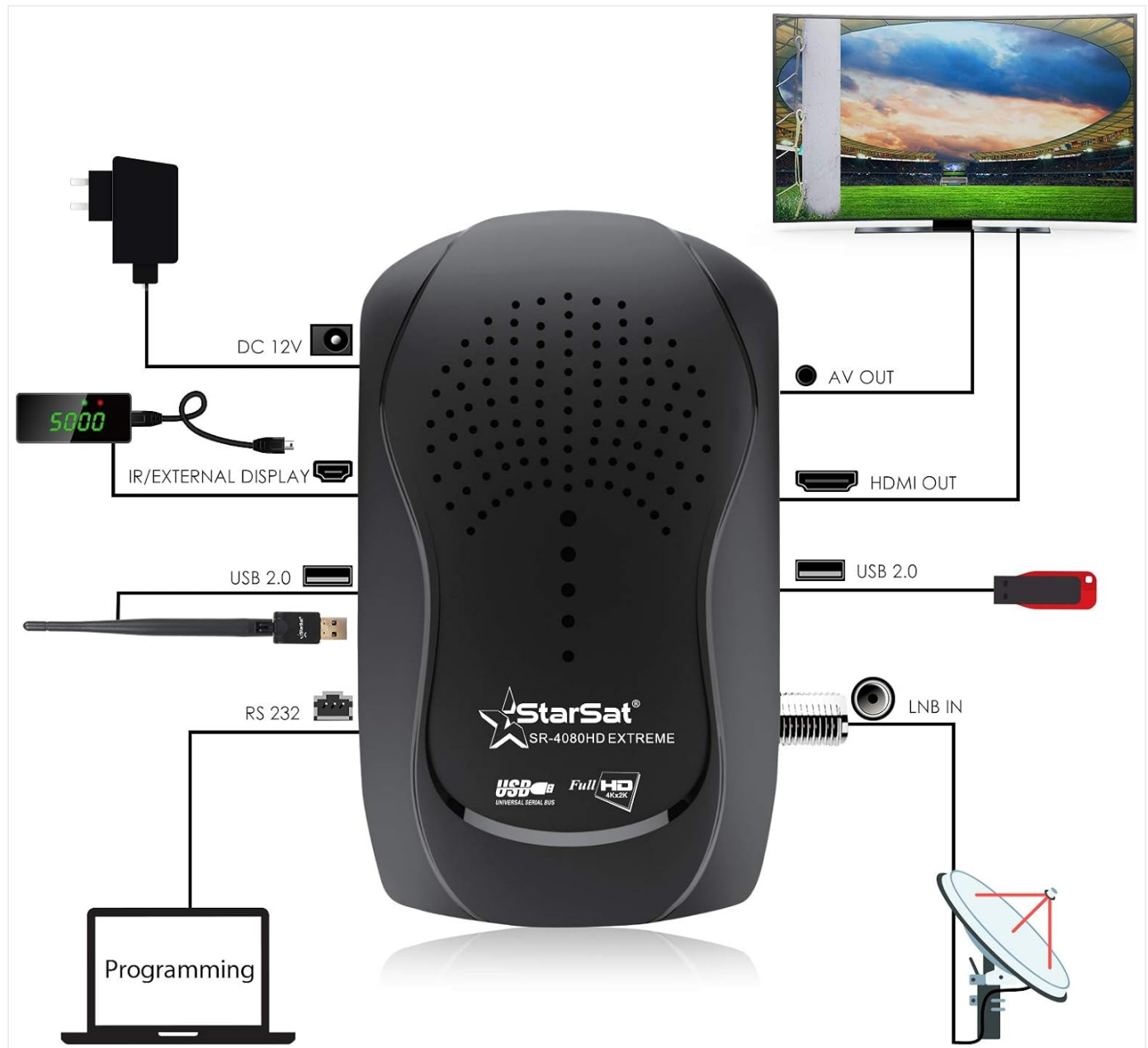
Figure 5.1: Visual guide for connecting the Star Sat SR-4080HD Extreme to a television and satellite dish, including power and peripheral connections.
