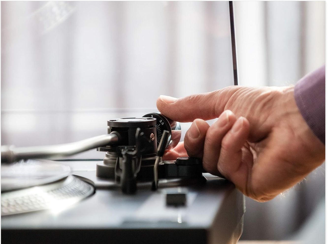
Figure 3: A hand adjusting the counterweight on the tonearm, a crucial step for proper tracking force.
