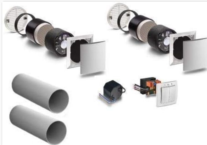
Figure 1: Exploded view of the Lunos e 2 decentralized ventilation units and accompanying accessories. This image shows two complete ventilation units, two round ducts, a universal control unit, a power supply, and a wall switch. Each ventilation unit consists of an outer grille, a fan, a ceramic heat exchanger, and an inner panel with a filter.
