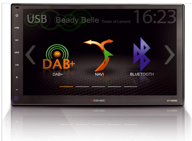
Figure 2.1: Main interface of the Z-N956, displaying quick access icons for DAB+, Navigation, and Bluetooth.
