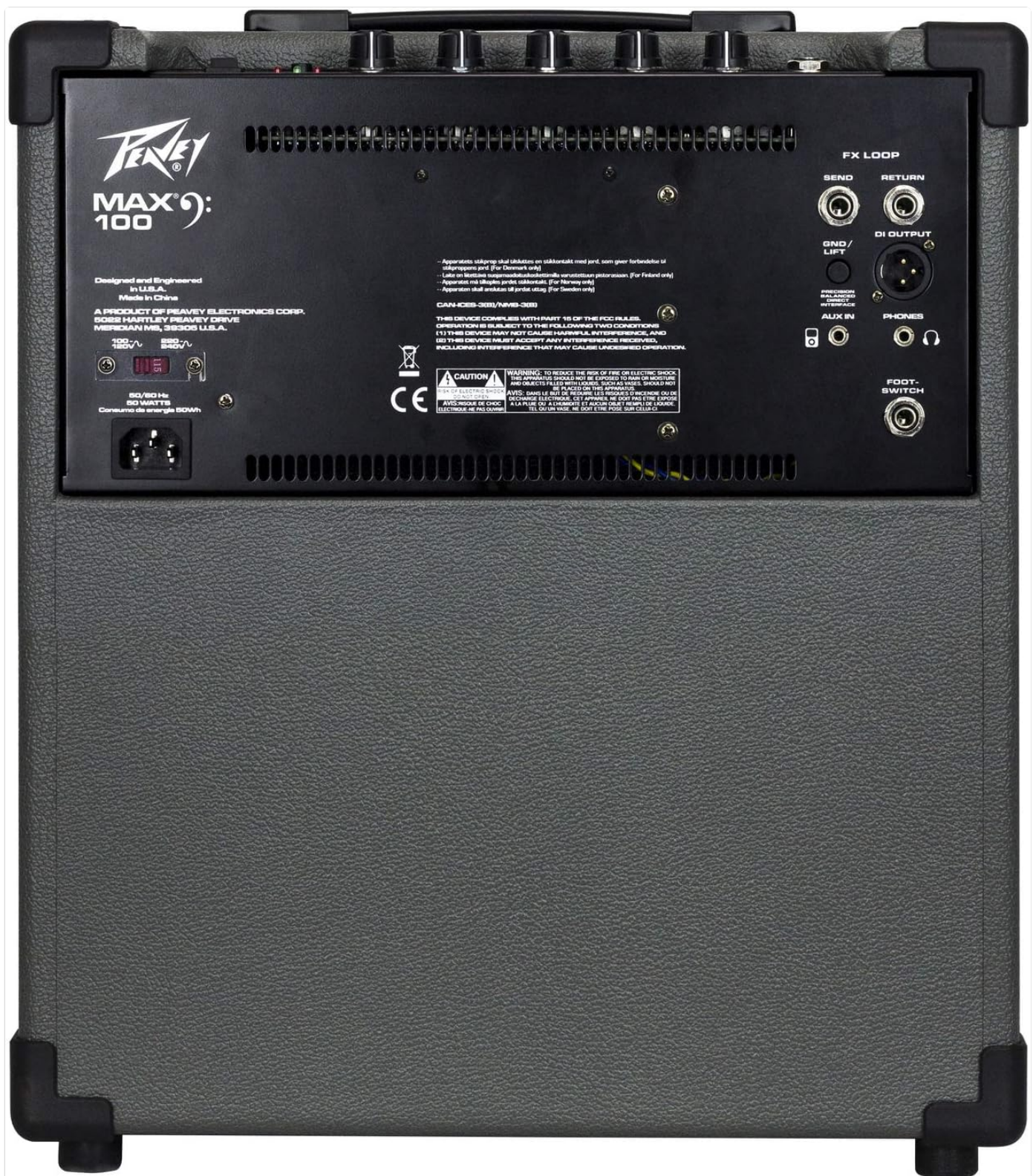
Figure 2: Rear panel of the Peavey MAX 100, detailing the FX Loop, DI Output, Aux In, Phones, and Footswitch connections.
