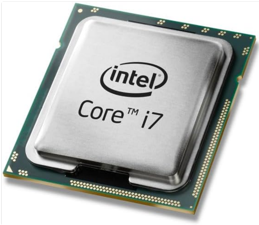
Image: The Intel Core i7-7700 processor chip, showing its metallic heat spreader and green substrate.
