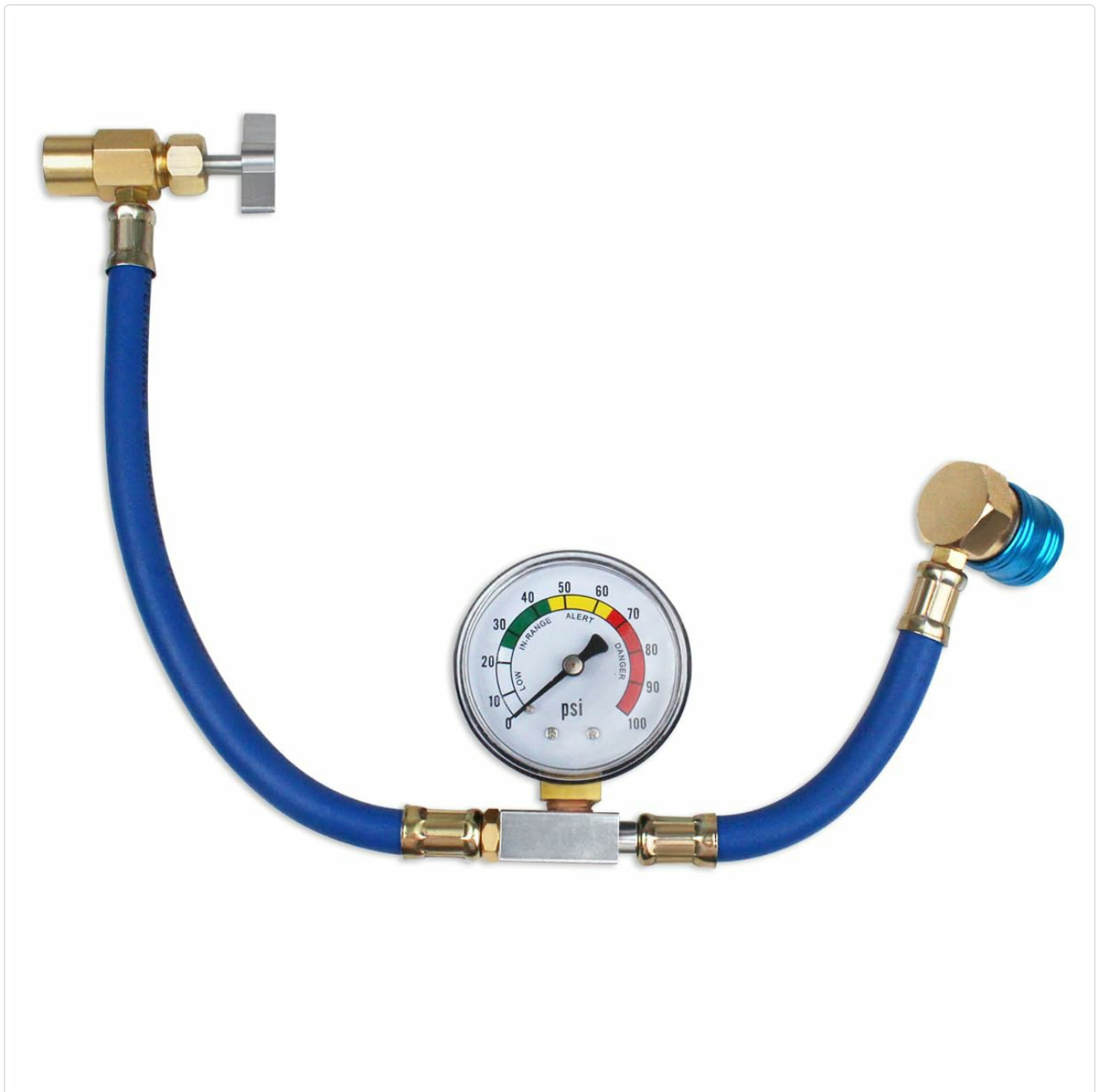
Figure 1: Pressure Gauge. This gauge displays the low-side pressure of your vehicle's AC system, with a scale from 0 to 100 PSI. It features color-coded zones for 'LOW', 'IN-RANGE', 'ALERT', and 'DANGER' to assist in proper charging.
