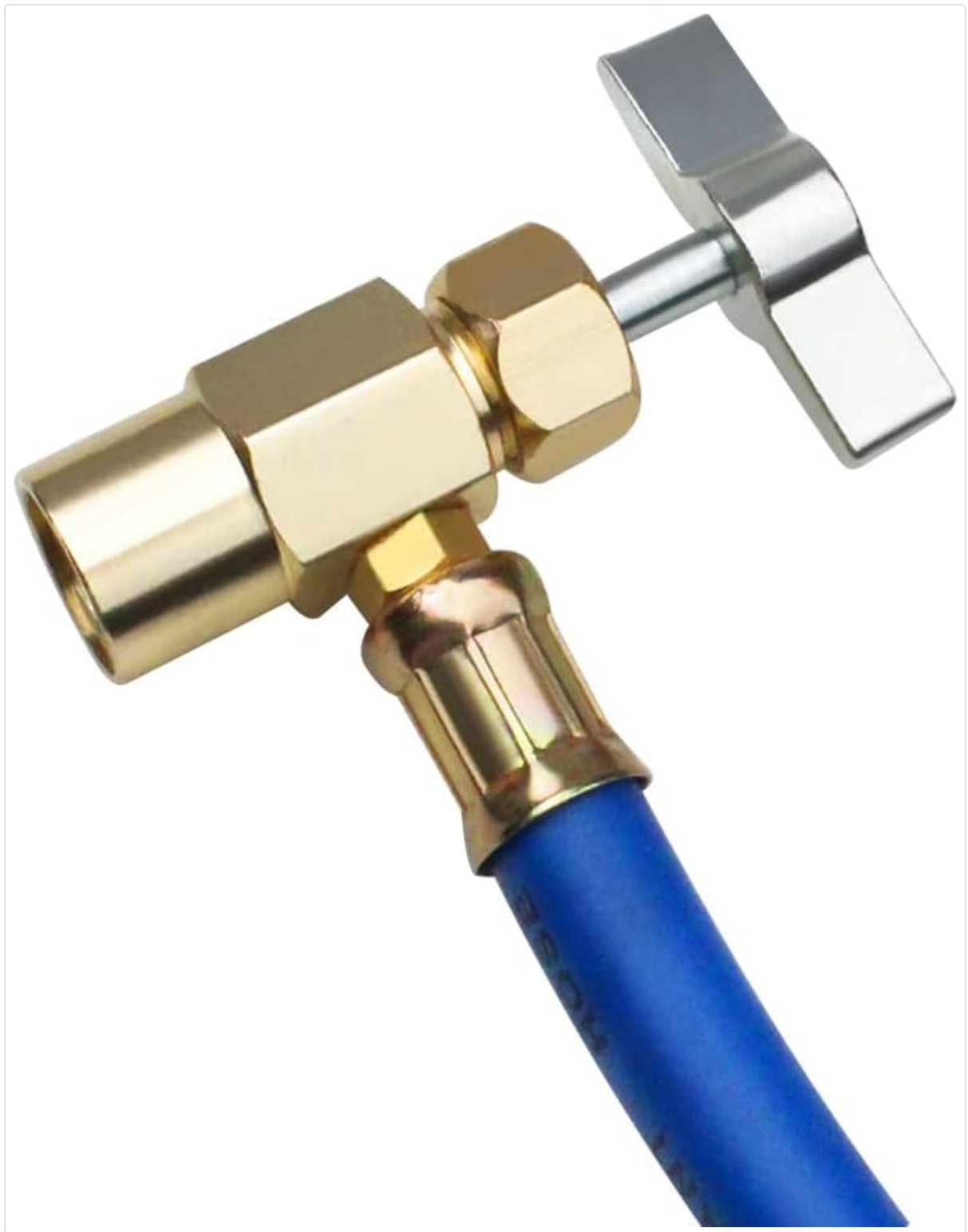
Figure 2: Refrigerant Can Tap. This component connects to the R134a refrigerant can. It features a 1/2" ACME fitting and a piercing needle mechanism to open the can and allow refrigerant flow into the hose.
