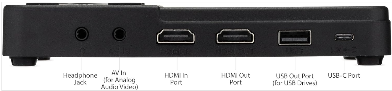
Image 4.2: Rear ports of the device, including Headphone Jack, AV In, HDMI In, HDMI Out, USB Out, and USB-C.
