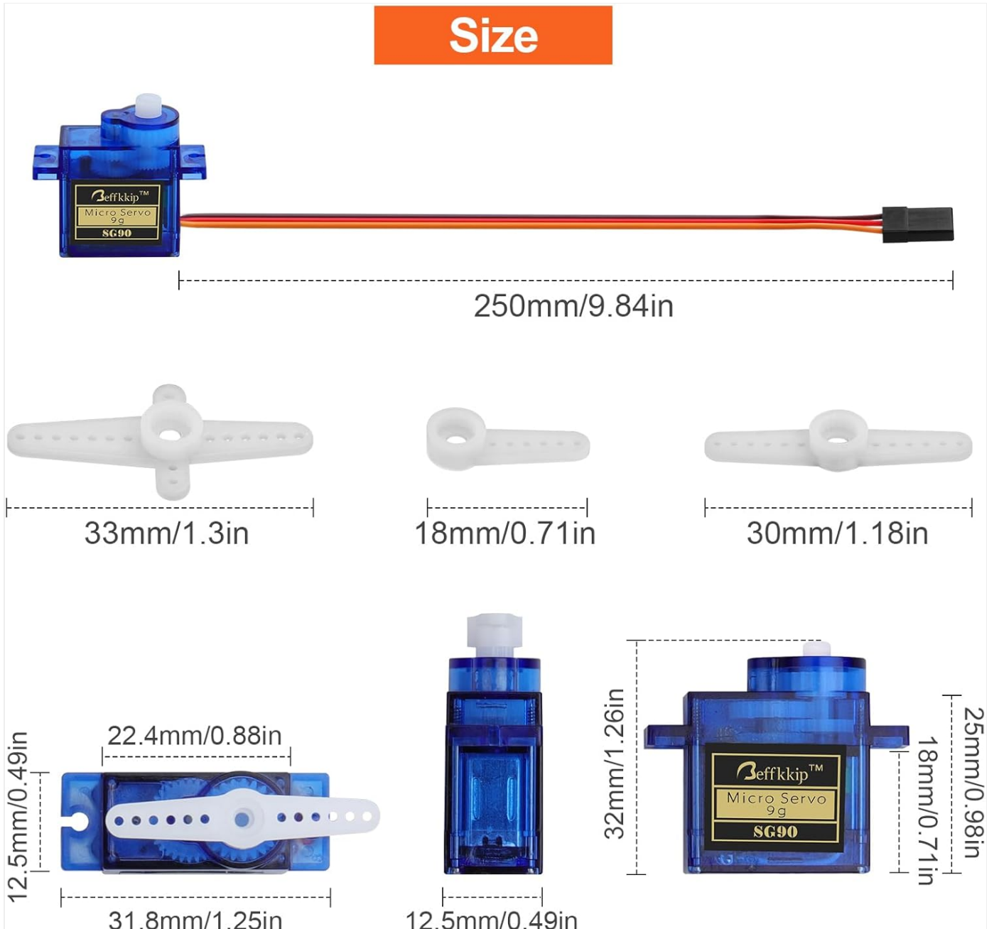
Figure 7.2: Detailed physical dimensions of the SG90 Micro Servo and its included horns.
