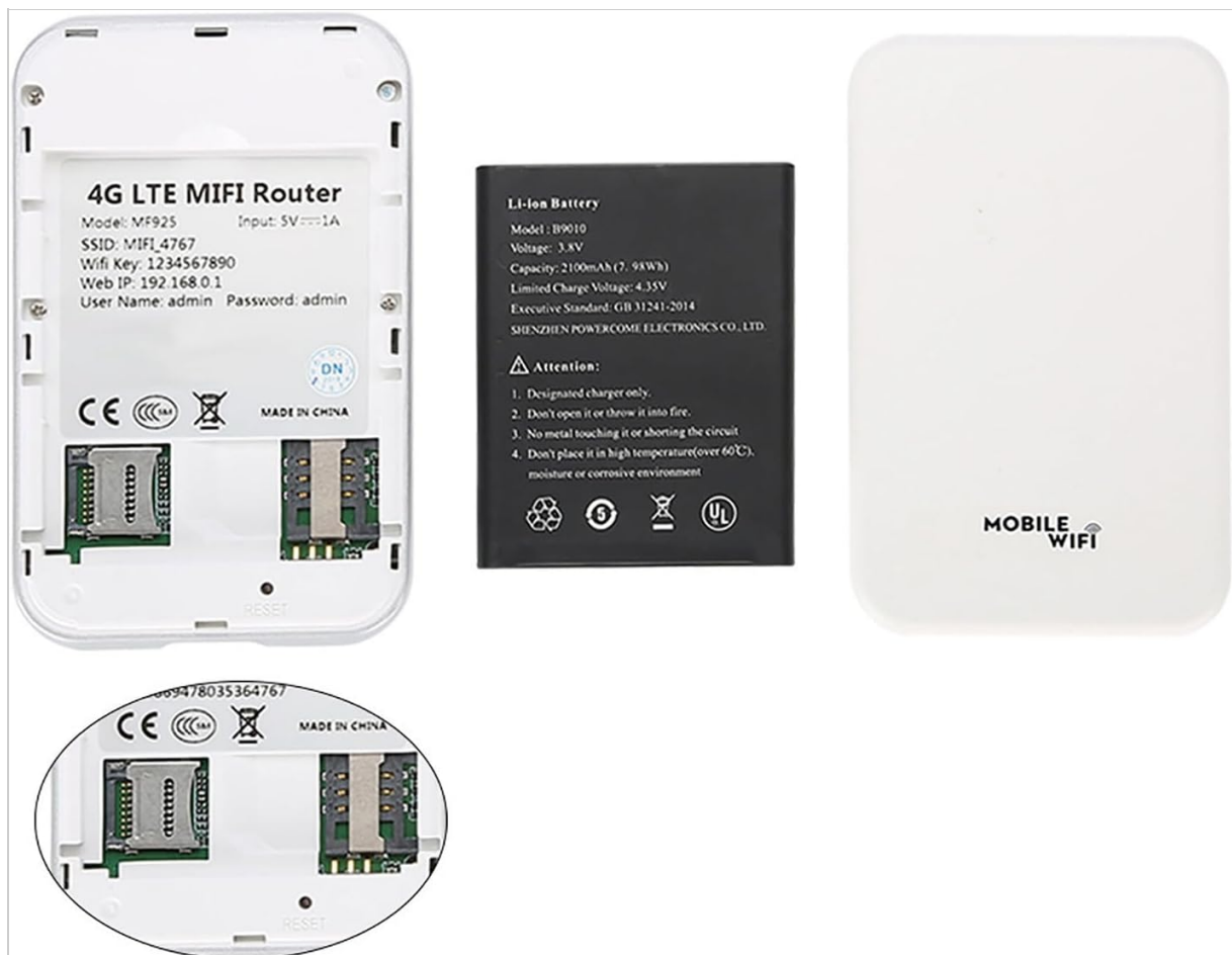
Figure 3.1: Internal view with battery and SIM/SD card slots.
