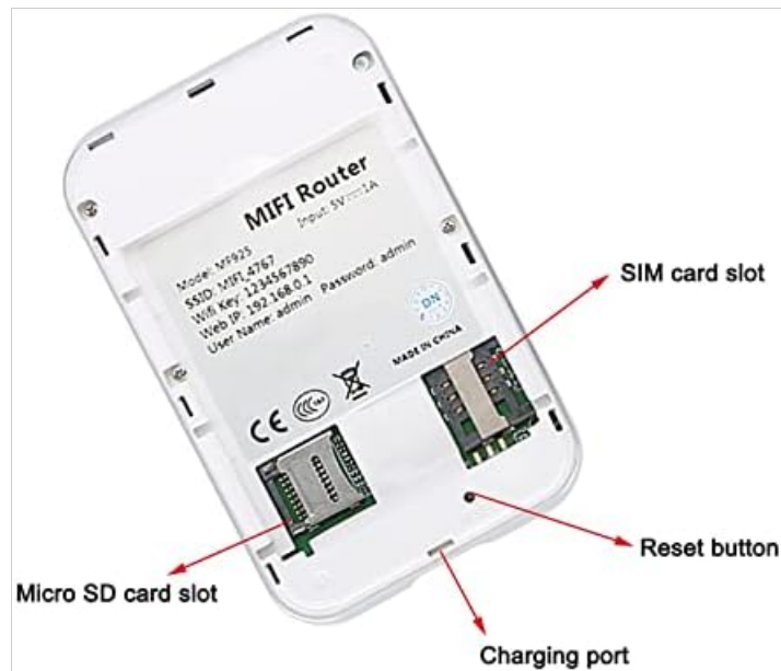
Figure 3.2: Detailed view of card slots and ports.
