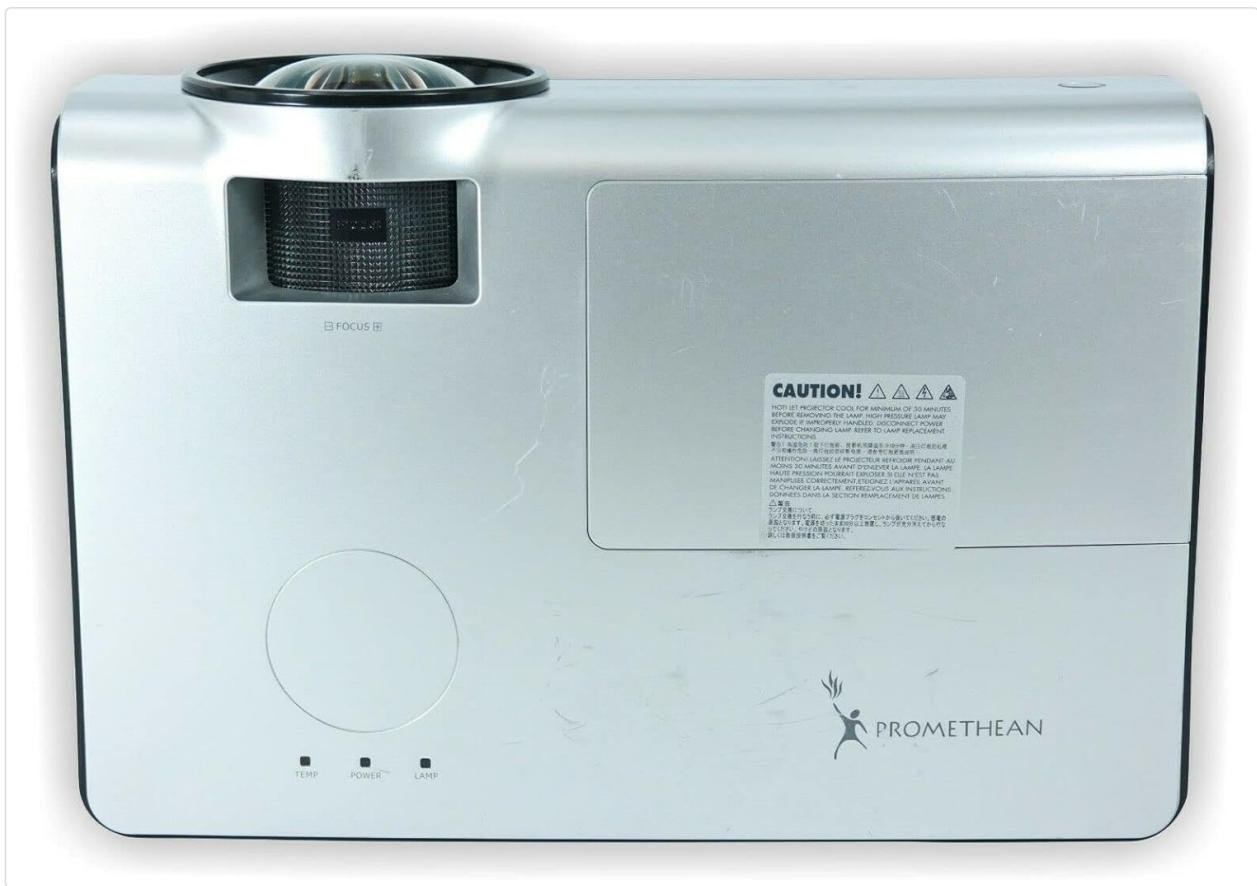
Image: Top view of the PROMETHEAN PRM-35 projector, showing the control panel area and lamp access cover. The top panel includes indicator lights for temperature, power, and lamp status, along with a caution label regarding lamp heat.
