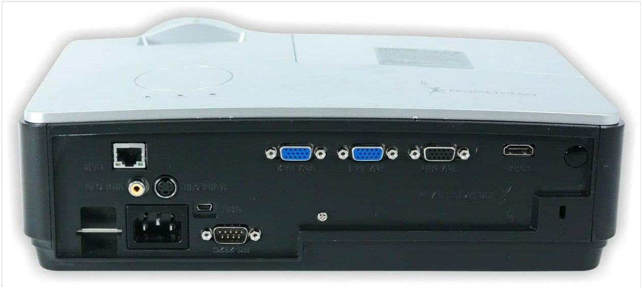
Image: Rear view of the PROMETHEAN PRM-35 projector, displaying a variety of input and output ports including HDMI, VGA, USB, S-Video, and network connections. The rear panel provides all the necessary input and output ports for connecting to various devices. These include HDMI, VGA, S-Video, USB Mini Type-A, RS232, RJ-45 (LAN), and audio jacks.
