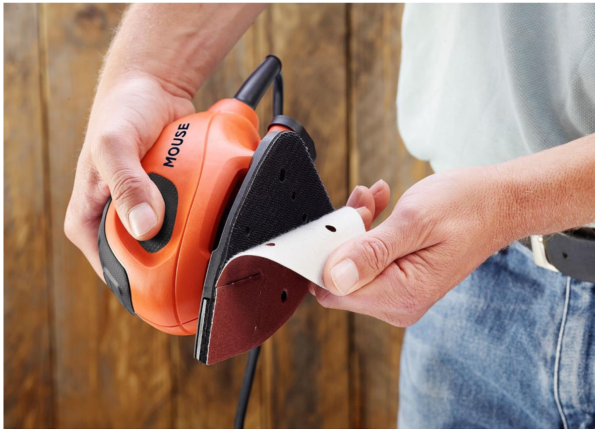
Image: A user demonstrating how to attach a sanding sheet to the base of the Mouse Sander using the Velcro system.
