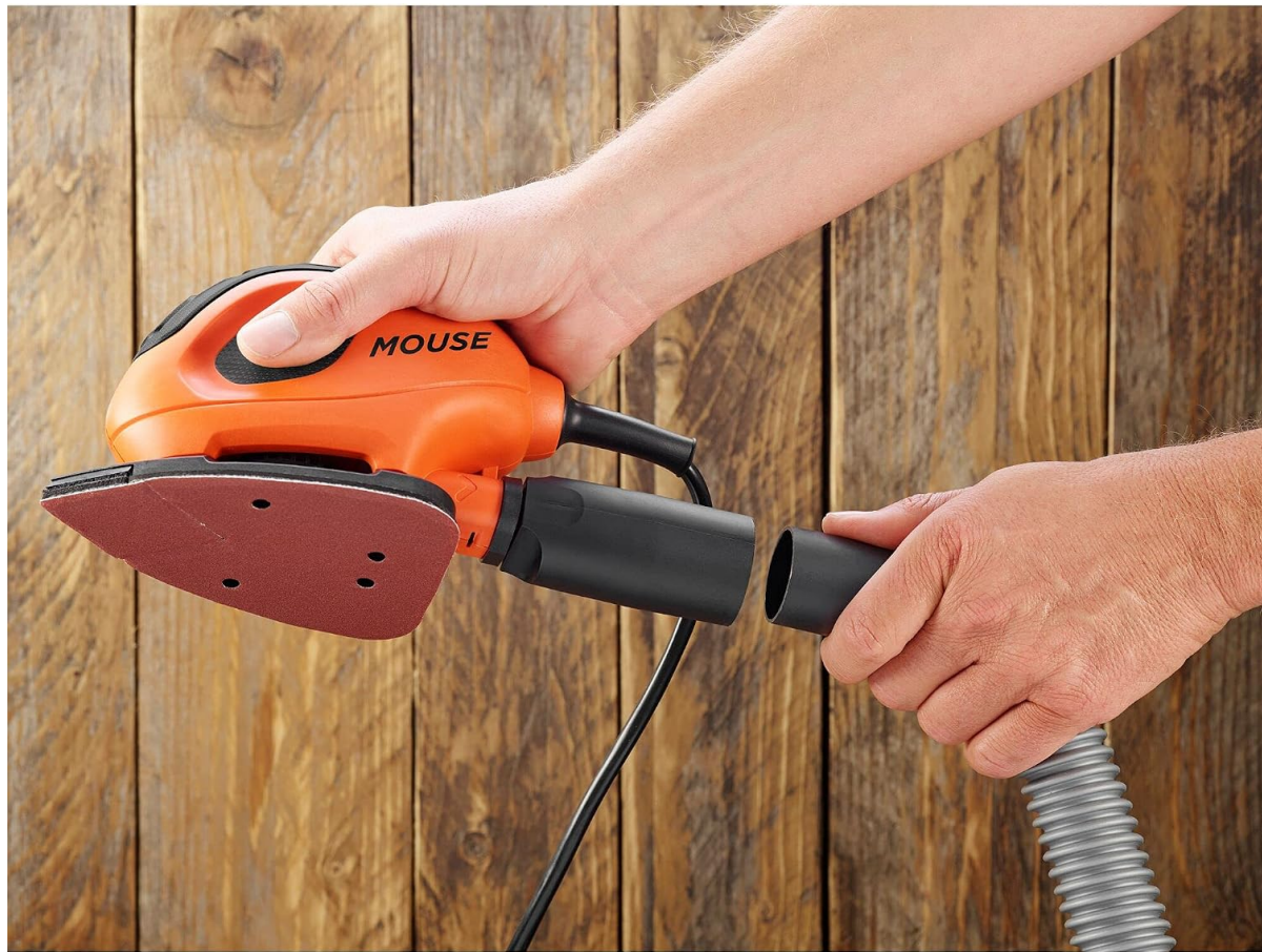
Image: A user connecting a flexible dust collection hose to the dust extraction port of the Mouse Sander.
