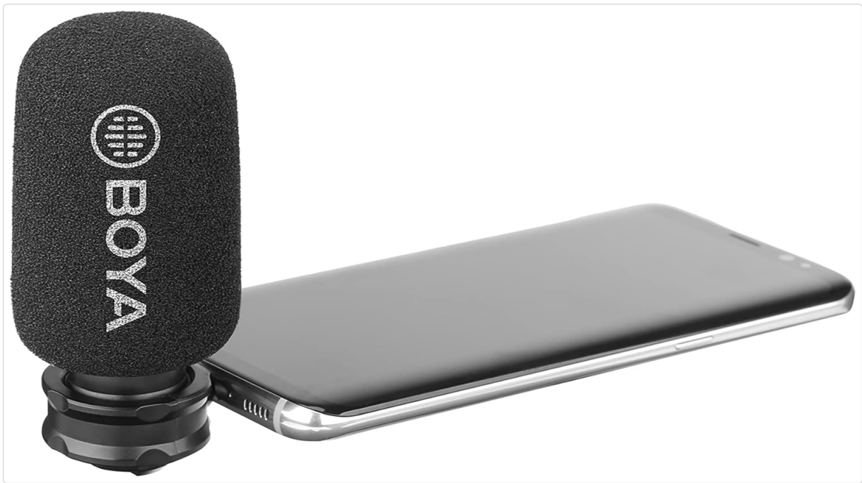
Figure 2: Microphone connected to an Android smartphone with foam windscreen.
